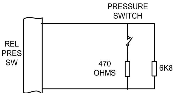
Figure 10. Example of wiring to a monitored input
