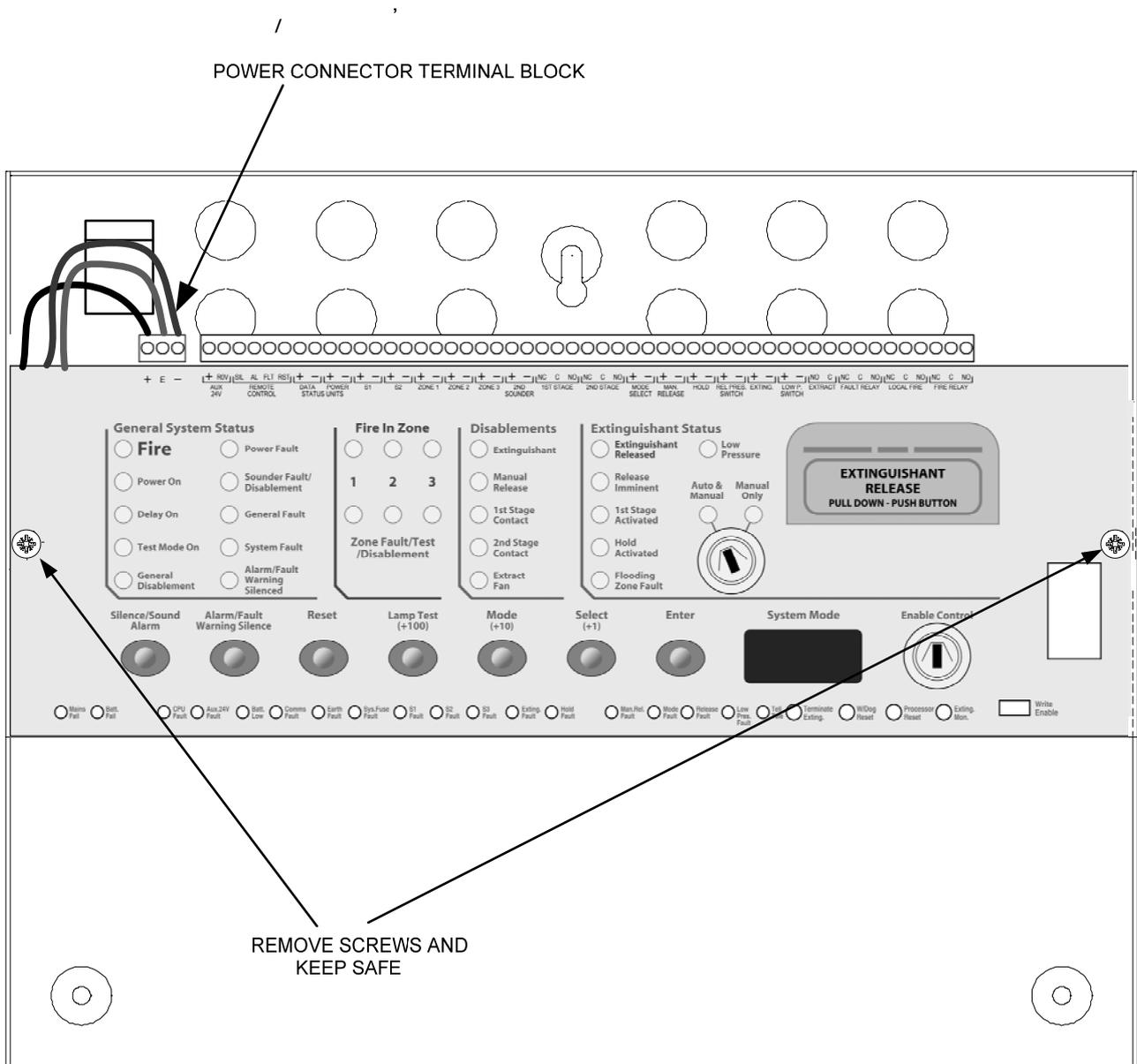
Figure 4. Removing the fascia
