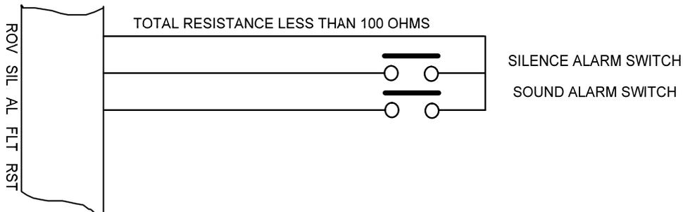
*Figure 14 - Example connections to remote control inputs*
