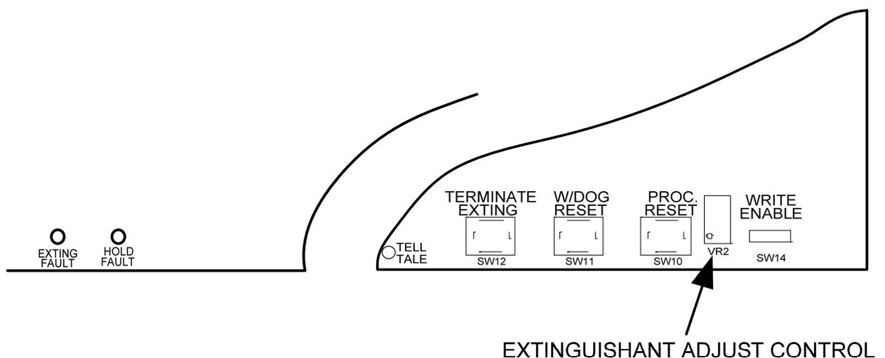
Figure 13. Extinguishant adjust control and Exting fault LED
