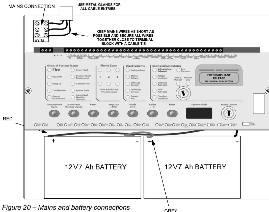
Figure 20 – Mains and battery connections
