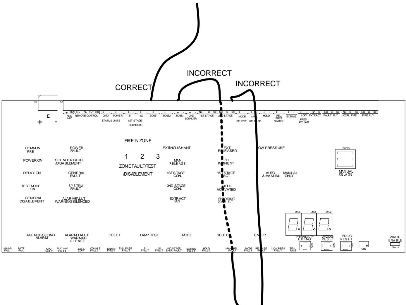
Figure 5 Wiring to the circuit board
