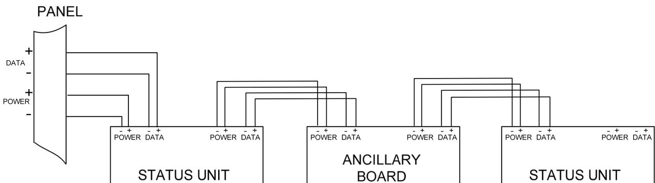
Figure 15. – Wiring to status units and ancillary boards
