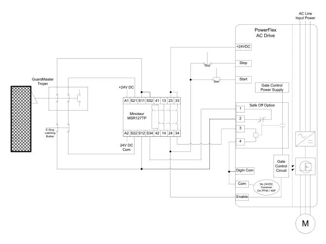
The gate will trigger the safety function. When triggered the safety relay outputs (Terminals 13 to 14, 23 to 24, and 33 to 34) open. This immediately removes +24vdc from the drives enable and Start/Stop inputs, and the Safe-off Option relay. The result is the drive is disabled, a stop signal is asserted, the Safe-Off Option goes to a safe state (off), and the motor will coast to stop. The Safe-off Option N.C. auxiliary contacts are monitored by the safety relay at terminals S52 & S34.
