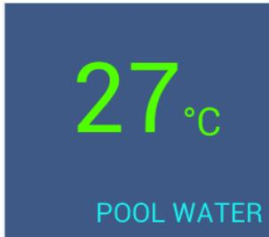
In this second part the actual pool temperature is shown. This value can be measured in different ways. This value will show standard the temperature the sensor at the heatpump measures. This sensor calculates the value of the water that flows into the heatpump. When the heatpump is not working, the value that was measured last when the heatpump was working will be shown.
