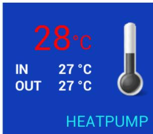
In the fifth part the divers temperatures will be shown. De big red temperature will show the temperature set (in this case: 28°C). Also the in and outgoing water temperatures will be shown, which will be measured at the heatpump. In the image are the in and outgoing temperatures the same (27°C).
