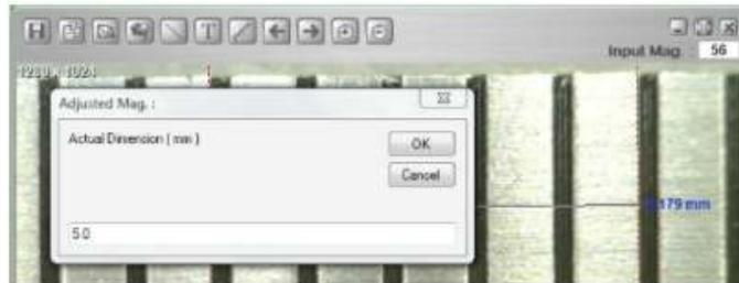
**Step 8:** The software will automatically calibrate the magnification rate and will show the adjusted magnification rate in the upper right corner of the picture.
