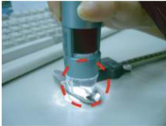
**Step 2:** To determine the magnification value of the image, refer to the reading on the center of the focus dial indicated by a small node. This is the magnification value for the captured image.
