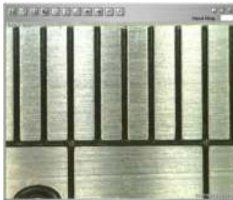
**Step 3:** Determine the magnification value from the reading on the DinoLite adjustment dial. Enter this value in the "Input Mag" box located in the upper right hand corner of the screen.
