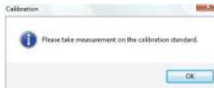
**Step 6:** Take a sample measurement of the selected calibration standard by clicking on beginning and ending points across a known measurement value (such as 5 mm, .5 in., etc.). A measurement value before calibration will be displayed (5.179 mm in the example below).
