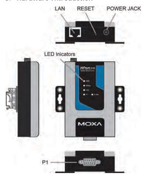
Reset Button—Press the Reset button continuously for 5 sec to load factory defaults: Use a pointed object, such as a straightened paper clip or toothpick, to press the reset button. This will cause the Ready LED to blink on and off. The factory defaults will be loaded once the Ready LED stops blinking (after about 5 seconds). At this point, you should release the reset button.
