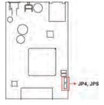
Jumpers are used to set the pull high/low resistors. The default is 150 K $\Omega$ . Short the jumpers to set this value to 1 K $\Omega$ . Do not use the K $\Omega$  setting with RS-232 mode, since doing so will degrade the RS-232 signals and shorten the communication distance.
