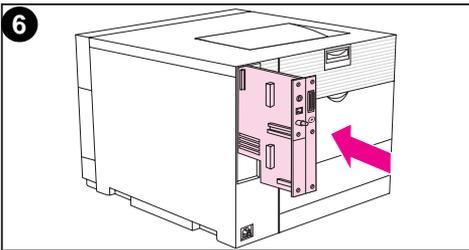
6 Insert the formatter board into the printer.
