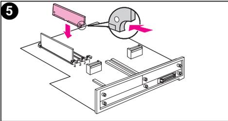
5 Align the connectors on the DIMM with the notches in the DIMM slot. Insert the DIMM into the slot and then firmly push the DIMM until the levers lock into place.
