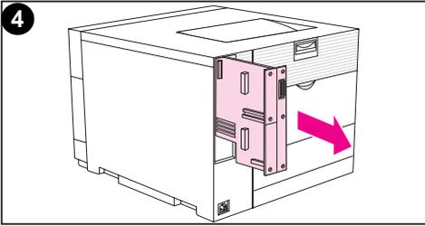
4 Slide out the formatter board and set it on a clean, flat, grounded surface.
