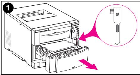
The toner density sensor should be cleaned whenever the imaging drum is replaced or whenever the control panel message DENSITY SENSOR OUT OF RANGE displays.
