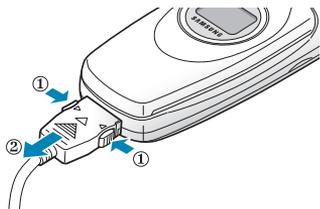
**Note:** Do not remove the battery from the phone without unplugging the adapter while it is charging. If you do this, the phone may be damaged.
