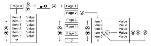
Press ESCAPE at any time in menu mode to step backwards one stage in the navigation process. Pressing ESCAPE when the page number is flashing will exit menu mode and return the display to normal operational mode; page 0.
