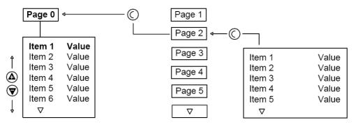
Press and hold RESET for two seconds at any time to immediately exit menu mode and return to the normal operational mode display. Any value or option adjustment that has not been confirmed and entered into memory will be abandoned and the original setting maintained.
