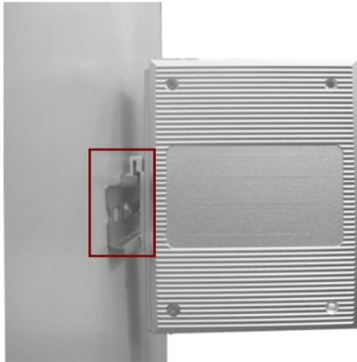
3. To remove the switch from the track, push downward on the unit to compress the spring, and pull the bottom outward from the track to disengage the unit and lift it off the track.
