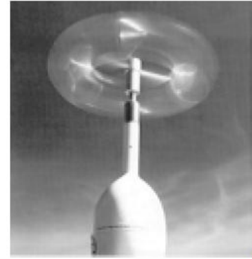
Figure BL.1: An anemometer measures the wind velocity; it is both a vertical axis and drag based design.
