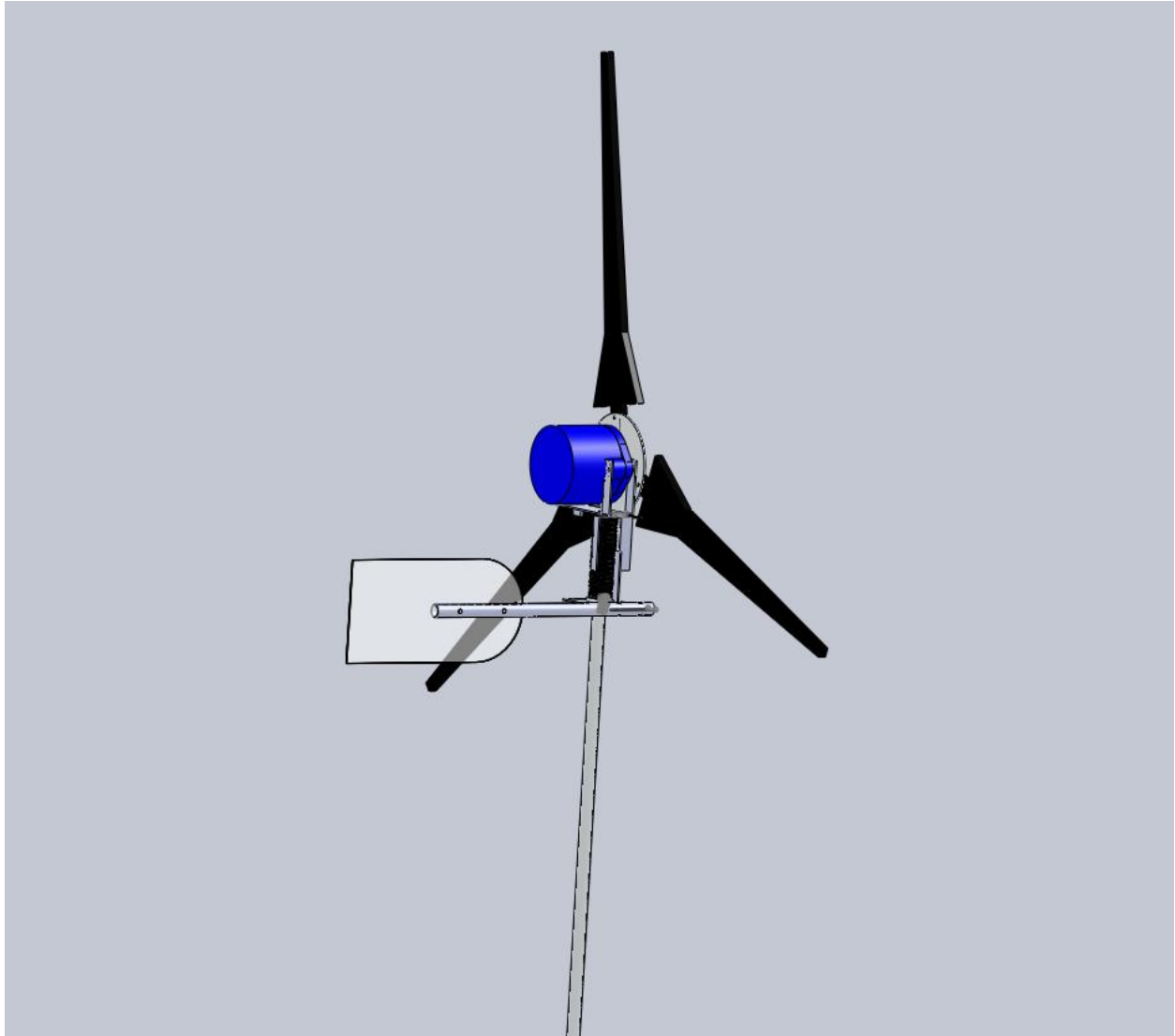
Figure F.11: The complete furling and directional fin subsystem.
