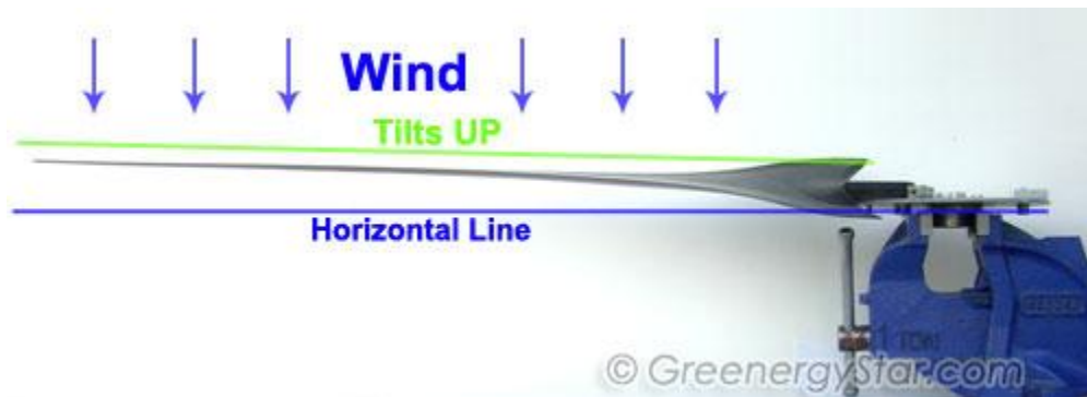
Figure BL.5: Forward-angled mounting of airfoil blades
