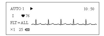
Under automatic mode, leads will be switched in order automatically while recording ECG. That means when ECG signal from one lead has been recorded for the set length such as 3 seconds, it will be switched to the next lead and begin recording another ECG signal. And there is a pause for several seconds before recording the next ECG signal under the modes of AUTO1, AUTO2 and AUTO3. Moreover, a 1mV calibration pulse will be printed on the record automatically before ECG of each lead.
