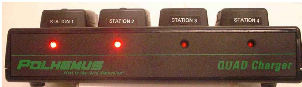
Figure 1-19: Standard Marker Batteries Charging
