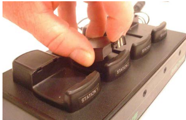
Figure 1-21: Standard Marker: Lifting The Battery
