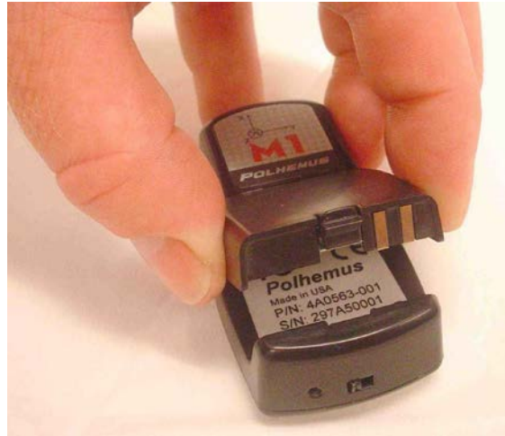
Figure 1-25: Standard Marker Battery Insertion
