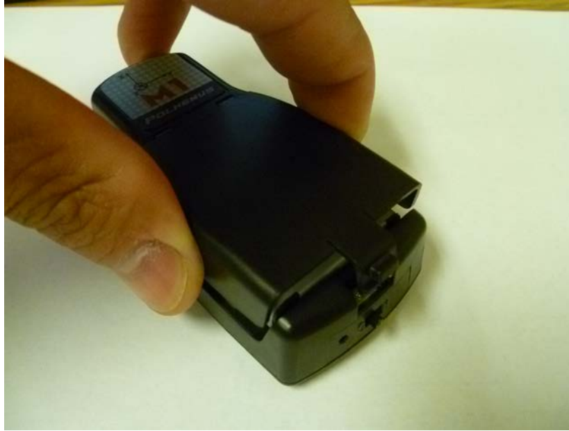
Figure 1-13 Extended Marker Battery Insertion
