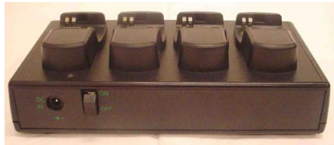
Figure 2-7: Standard Marker Battery Charger and Power Pack, Rear View
