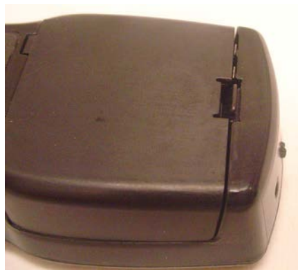
Figure 1-23: Standard Marker: Proper Seating Of Spring Clip
