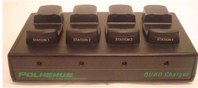
Figure 2-6: Standard Marker Battery Charger, Front View
