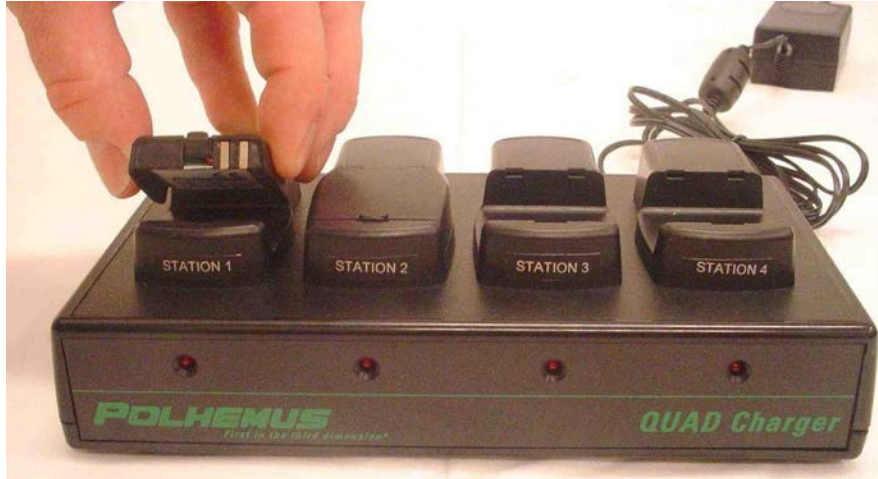
Figure 1-17: Standard Marker: Placing Batteries Into Charger
