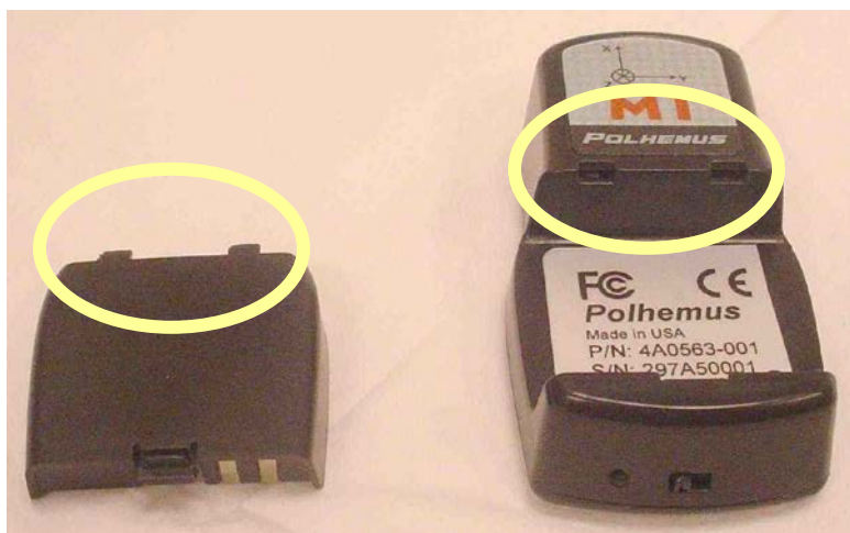
Figure 1-24: Standard Marker Battery Tab Orientation
