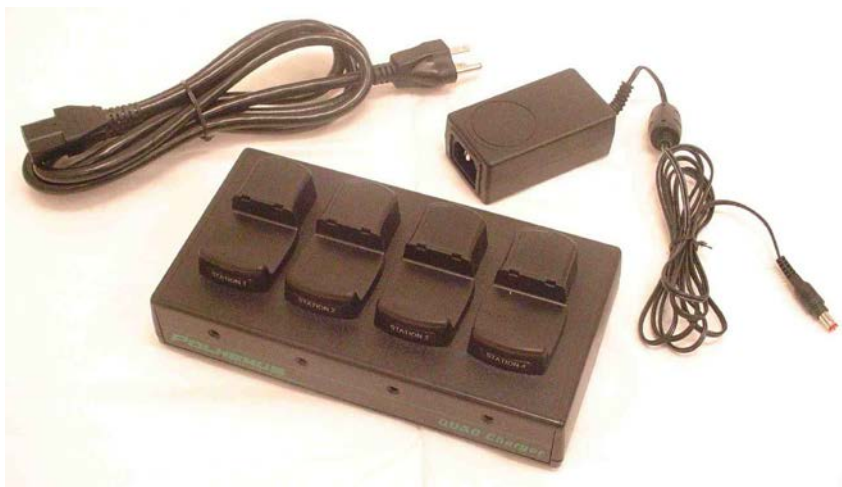
Figure 1-16: Standard Marker Battery Charging Components
