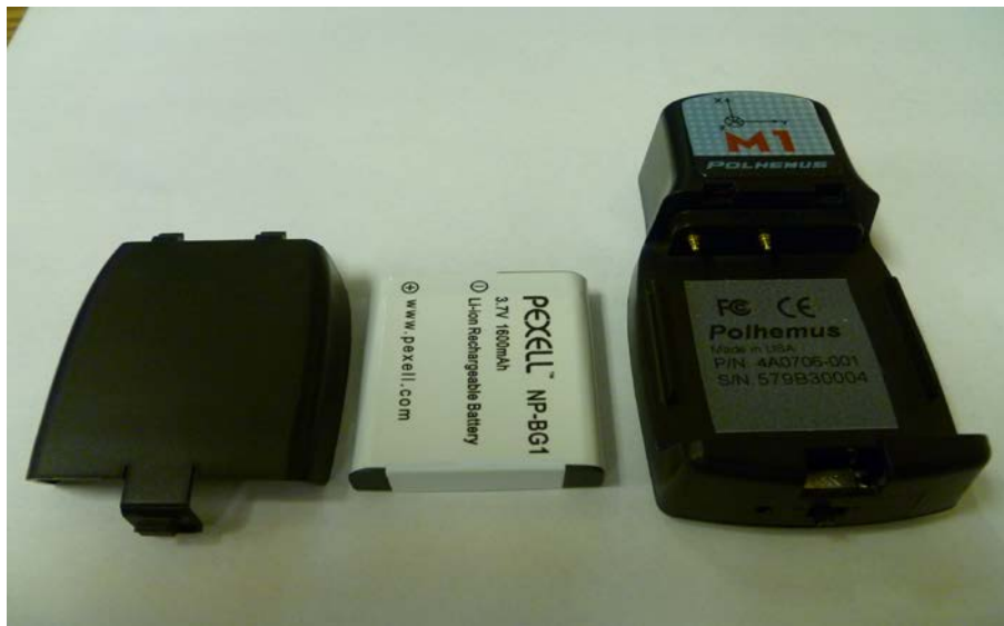
Figure 1-12 Extended Marker Battery Tab Orientation
