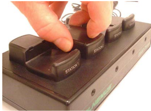
Figure 1-20: Standard Marker: Preparing To Remove The Battery
