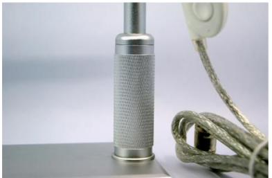
And the pen microscope can be move up and down by turning the pillar (see left photo) for getting larger photo area or smaller photo area.
