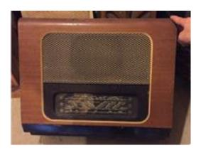
The set was capable of receiving short, medium and long wave bands. It had an internal 8" paper cone loudspeaker. Internally the components were mounted on a blue painted steel chassis.
