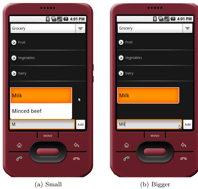
Figure 5.1: Normal autocompletion behavior, and the bug that appears after typing more letters. Notice how the autocompletion list hovers in mid air.
