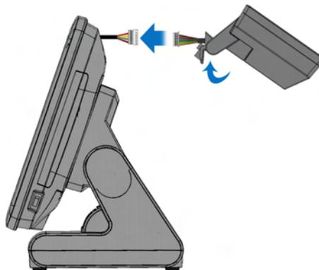
3. Mount the customer display to the device and tighten the two PHILLIPS M3 screws as shown below.
