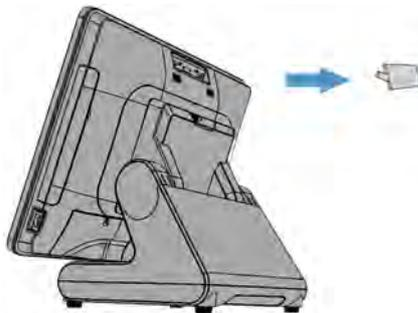
2. Adjust the hinge of the customer display, and then connect to the device as shown below.
