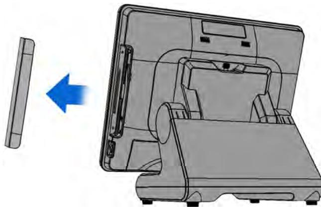
2. Connect the cable of the MSR assembly to the device.
