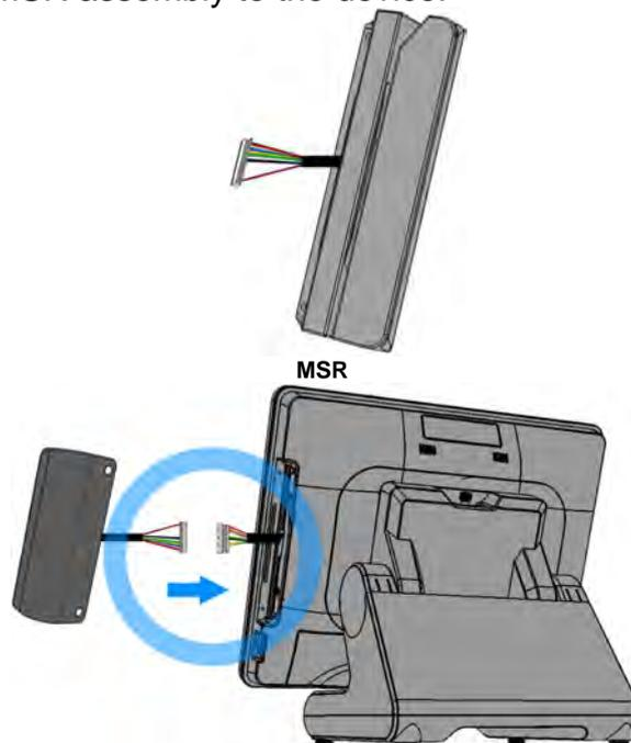
3. Tighten the two PHILLIPS M3 screws to fix the MSR assembly as shown below.
