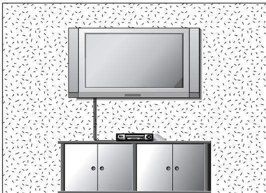
For proper ventilation, allow a clearance of 4" on each side and 2" from the wall. Detailed installation instructions are available from your dealer, see the optional Wall Mounting Bracket Installation and Setup Guide.
