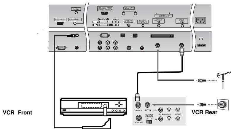
5. Antenna and Cable Service with a Cable Box
