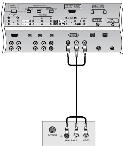
The TV has a special signal output capability which allows you to hook up a second TV or monitor.
