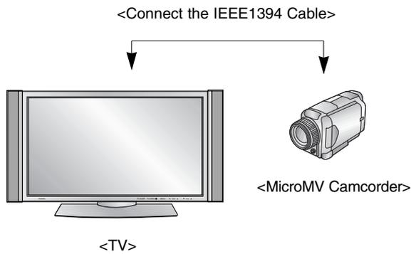
2. When connecting the DVHS and the MicroMV Camcorder, as shown in the (c) figure, press the **1394** button to show the contents panel and then select the DVHS or the MicroMV Camcorder to show the control panel.
