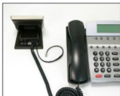
Connect the handset cord to the handset port on the Soundshield with the handset symbol.
