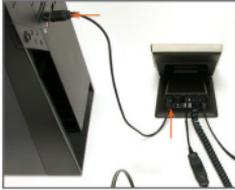
To power your Soundshield, connect the USB Cable to the USB port on the back of the Soundshield and connect the USB cable to your PC.
