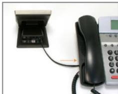
**Note:** The Soundshield tail cord is already connected to the Soundshield's telephone port.
