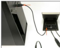
To power your Soundshield, connect the USB Cable to the USB port on the back of the Soundshield and connect the USB cable to your PC.
