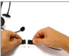
Connect the bottom cord (curly cord) to the Headset port of the Soundshield with the headset symbol.
