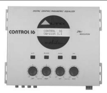
Input Gain Controls: Use these controls to match the pre-amp output level from your car audio source unit. Set the input level so that the SIGNAL LED (next to the input sockets) lights occasionally on musical peaks. Control16 MAX Input level: 15 V
