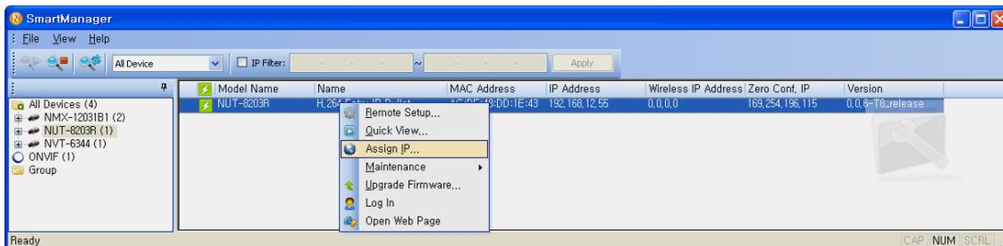
4. Select Assign IP. You can see a Assign IP window. Enter the required IP address.
