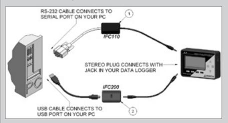
1. Fully insert the male connector of the IFC110 interface cable into the female receptacle of the data logger. Insert fully the RS232 connector into the Serial Port.
