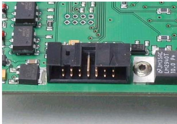
The JTAG connector is used for programming the microcontroller at the factory. If you are intending to re-program the device in the field please contact Sensor Line GmbH for further information.
