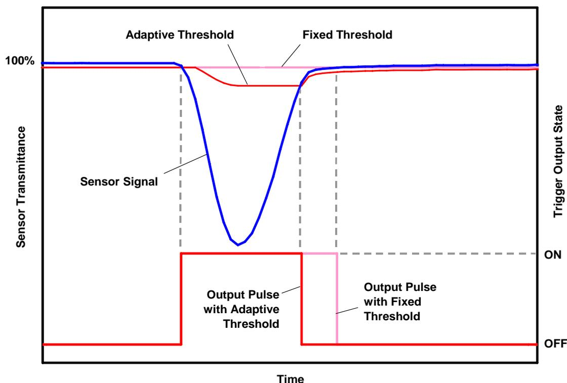
Adaptive threshold processing can be switched on and off. The ratio of signal amplitude to which the trigger threshold adapts can be defined to values of 50%, 25%, 12.5% and 6.25%. Please refer to section 3.2.4 for instructions.
