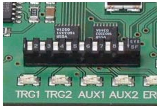
The SIL switch consists of eight individual switches which are connected to I/O pins of the microcontroller. They are used to signal different conditions in order to modify the behavior of the interface without re-programming it. Please refer to the software section of this manual for the different switch settings.
