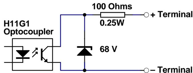
The above schematic shows the internal circuitry of the TRG1 & 2 and AUX1 & 2 optocoupler outputs. When the phototransistor is illuminated by the LED (ON condition) current flows into the + terminal and out of the - terminal. The resistor limits the maximum allowable current to 50mA. Therefore, any DC voltage applied directly to the outputs must not exceed 5V when the phototransistor is conductive because the maximum power the 100 Ohm resistor can dissipate is 250mW.
