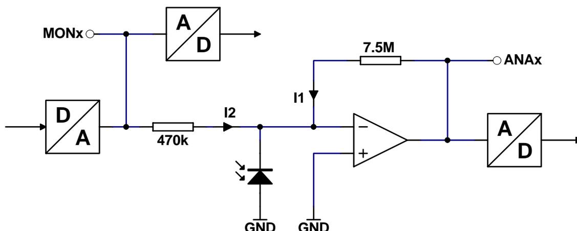
The drawing above is a simple circuit diagram of one channel. When the photodiode is illuminated with light from the sensor it proportionally sinks a current to the incoming light power. This causes the output of the OP to go high so the current is supplied across the 7.5M resistor. When the light becomes too bright the OP output is clipped, and the controller supplies additional current via the DAC and the 470k resistor until the OP output is "unclipped."
