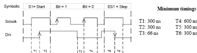
Figure 22. start of frame, a one, a zero and the end of frame [8].
