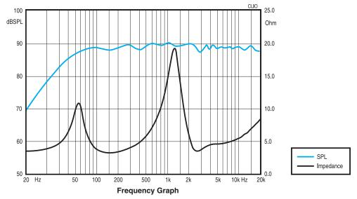
Specifications: • Impedance: 4 ohms • Frequency response: 38 - 20,000 Hz • SPL: 89 dB 2.83V/1m • Power handling: 140 watts RMS • Traditional cabinet dimensions: 22" H x 9" W x 13.5" D • Curved cabinet dimensions: 22" H x (9" front, 4.5" back) W x 14.8" D.
