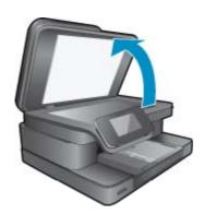
**b**. Load original print side down on the right front corner of glass.
