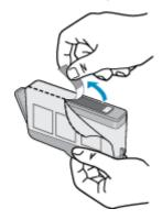
**b**. Twist orange cap to snap it off. A forceful twist may be required to remove cap.
