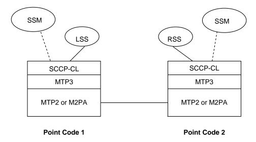
Figure 1. Necessary SS7 layers when running SSM
