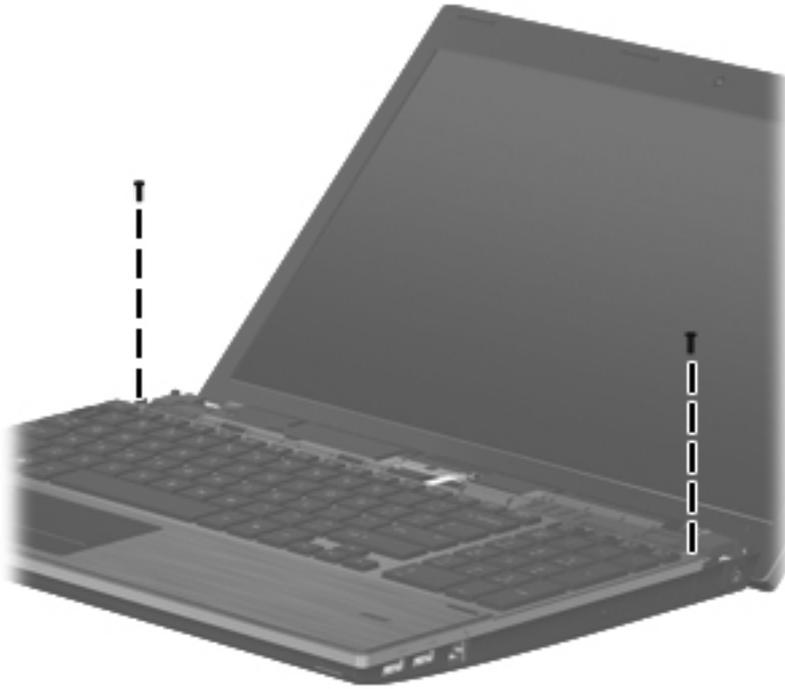
6. Slide the keyboard back toward the display **(1)**, and then rotate it forward **(2)** until it rests upside-down on the palm rest.
