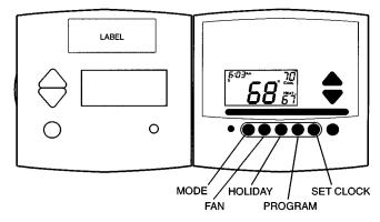
Fig. 3 — Thermostat Programming Buttons
