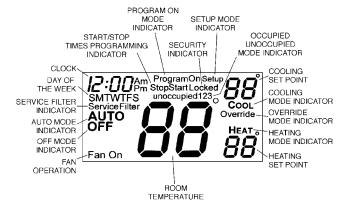
Fig. 1 — Thermostat Display
