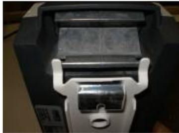
**Not attached properly.** Note the white bracket is in front of silver clip, which will not allow for an electrical connection.
