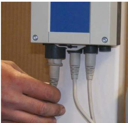
Locate the 24V Battery, the Battery Charging unit and the Handset Control. Charge the battery for 24 hours (see page 16 “Charging the Battery”) then install it on the bracket above the Control Box as shown above and in the photo to the left. Plug the Handset Control into the Control Box as shown above and in the photo to the left. Press firmly to make sure the plug is fully seated as shown below.
