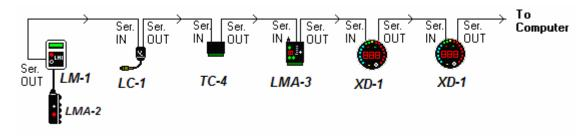
Devices attached to the LM-1's analog input count as being part of the LM-1's 6 channels. They don't count extra. XD-1's do not contribute any channels, so you can add as many as needed.
