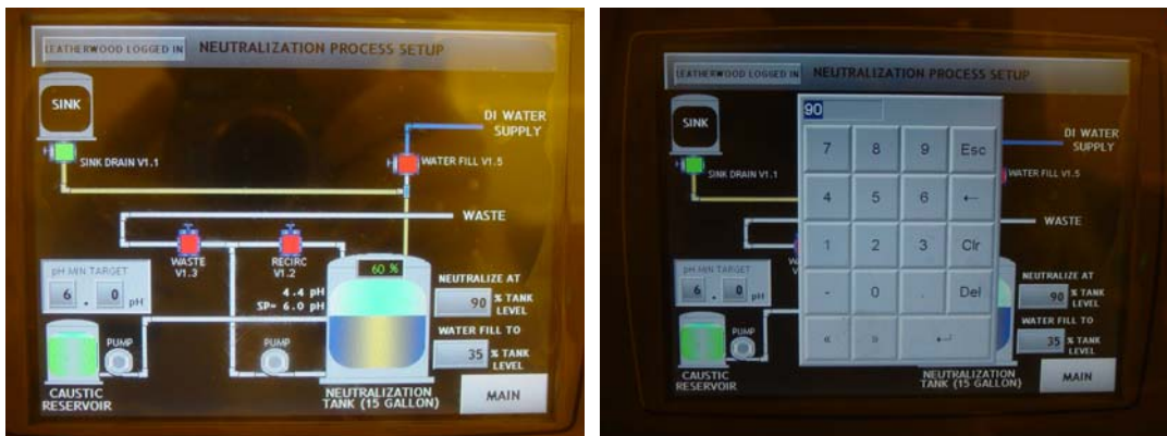
Figure B6. Neutralization Process Setup screen showing full screen (Left) and Pop-Up window for entering data (Right).
