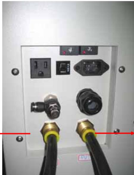
Water in connector on laser tube
