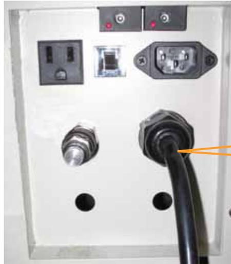
O ring B to fix the wiring
