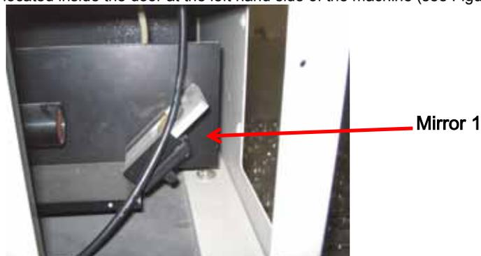
(Figure 8- 1 Cleaning the Mirrors)
