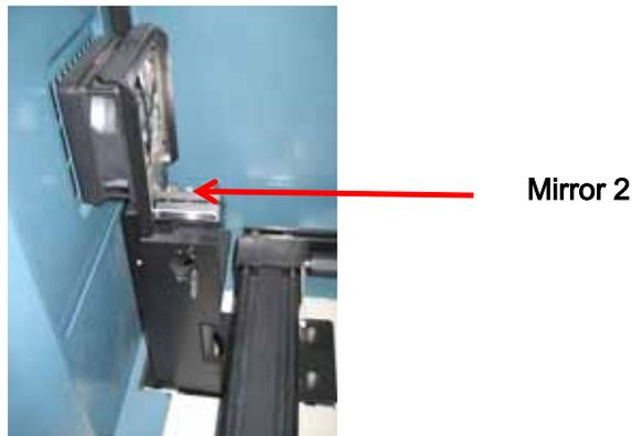
(Figure 8- 2 Cleaning the Mirrors)
