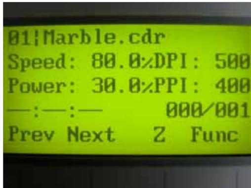
The main work page is the page that the LaserPro Gaia will default to upon startup and will be the “home base” for when navigating through the various functions of the control panel. This will be the page that is displayed when you are processing your jobs. This page contains specific job information such as the current job’s name, Speed, Power, PPI, DPI, processing / remaining times, and jobs loaded.
