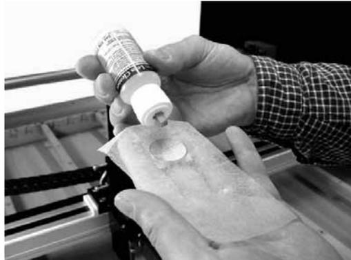
(Figure 8- 5 Cleaning the Mirrors)
