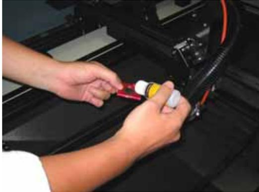
(Figure 8- 9 Cleaning the Focus Lens)
