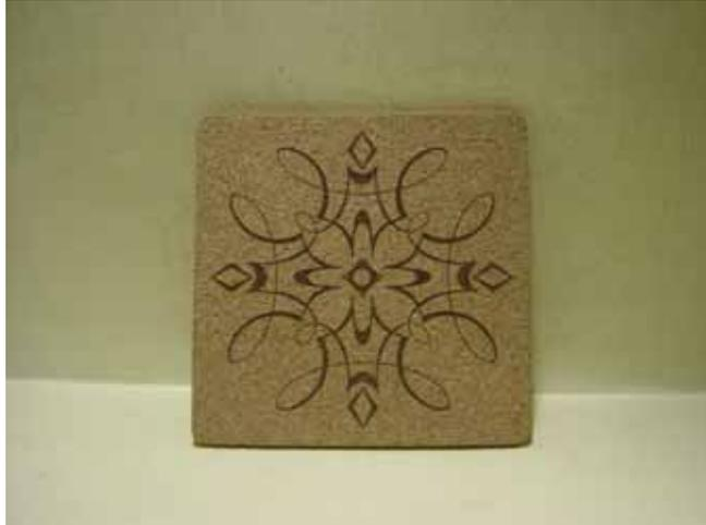
In these situations when there are raster engraving and vector cutting operations on a single project, the LaserPro Gaia driver will interpret between raster sections and vector sections by the types of lines and line widths of your design. Areas of your design with line widths set between 0.001" (0.025mm), 0.004" (0.1mm) will be designated for vector cutting, and the other areas will be designated for raster engraving.
