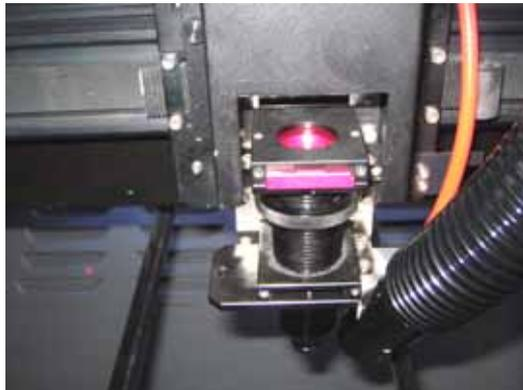
(Figure 8- 8 Cleaning the Focus Lens)
