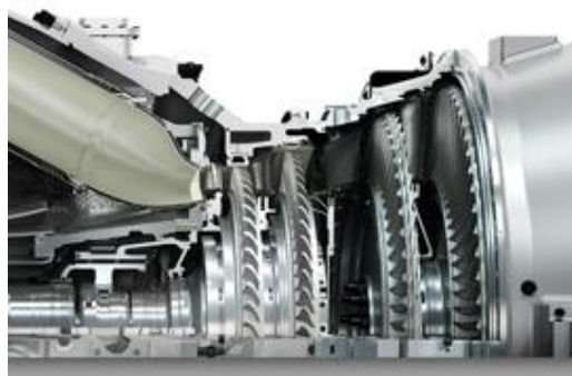
Figure 2.5 Turbine section after the combustion chamber ; Hellberg (2011)
