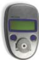
▲ Newer prototype diffusion porometer based on the same principles as the 1970s prototype but with modern electronics.
