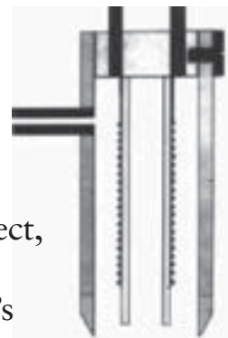
▲ Ellis Wallihan's porometer design with the Dunmore electronic humidity sensor (circa 1960.)
