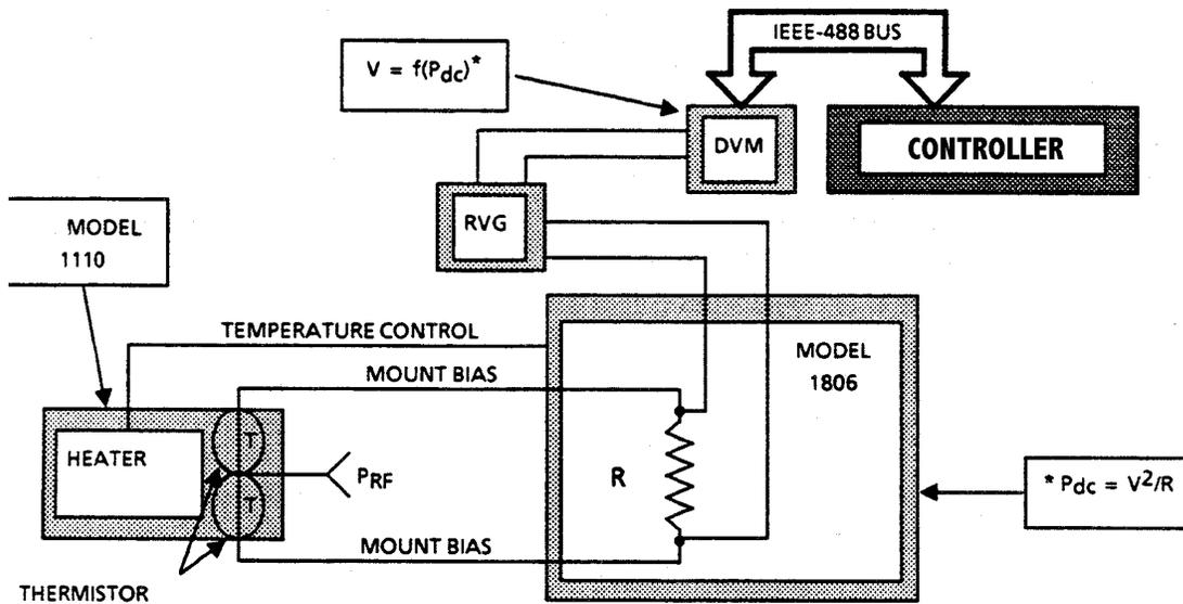
Figure 4-1 Functional Block Diagram of Precision Power Measurement System
