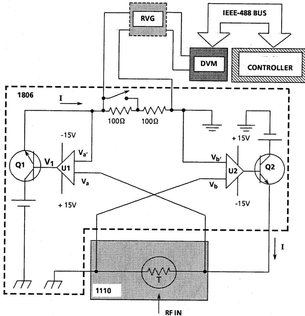
Figure 4-2 Simplified Schematic of Precision Power Measurement System
