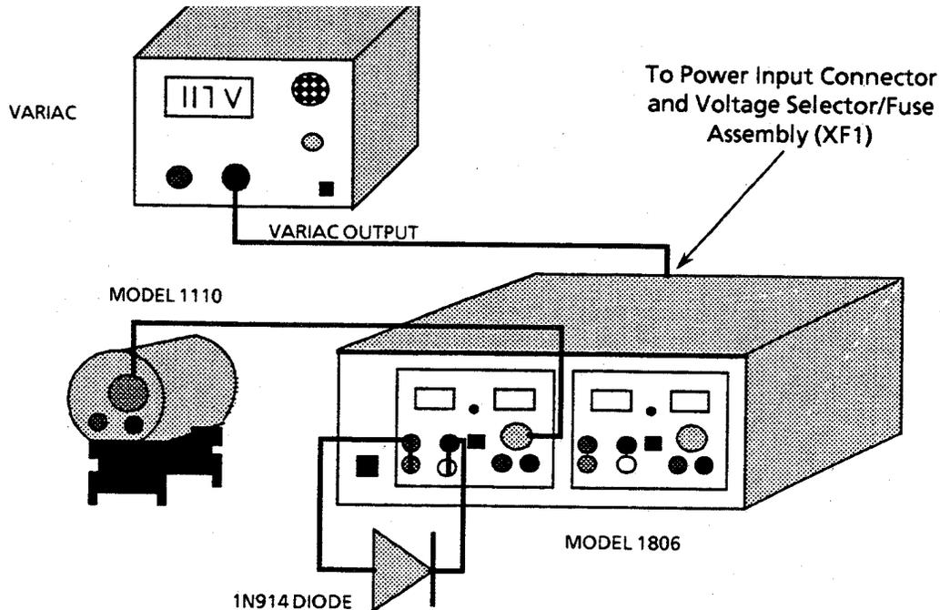
Figure 5-5 Initial Test and Calibration Configuration
