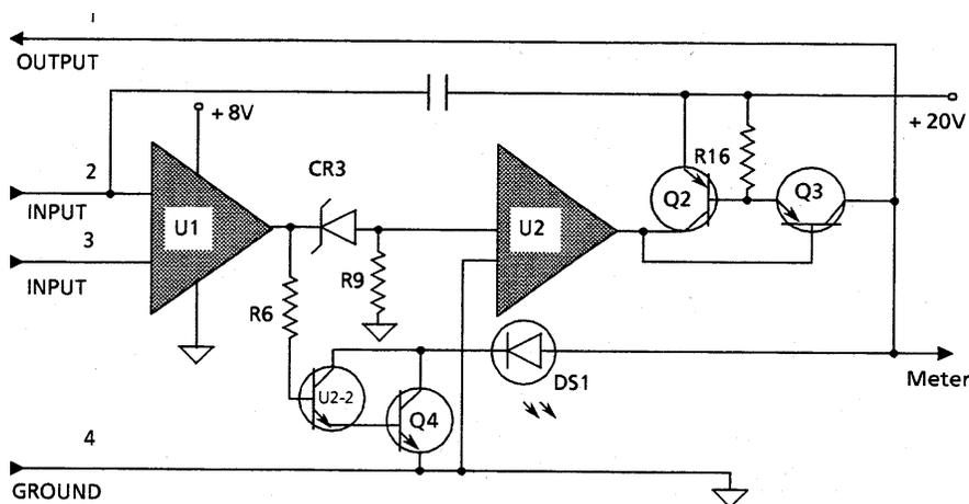
Figure 4-3 Simplified Schematic of Model 1806 Temperature Control Board
