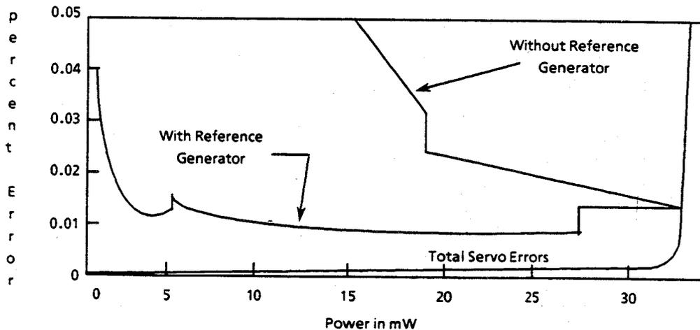
Figure 4-5 Graph of Typical Bridge Errors With and Without Reference Voltage Generator<sup>1</sup>
