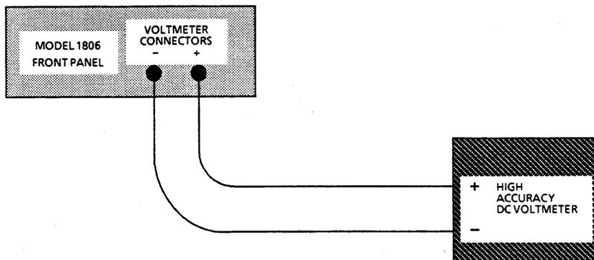
**Figure 3-2 Location of Digital Voltmeter in Typical Test Configuration**
