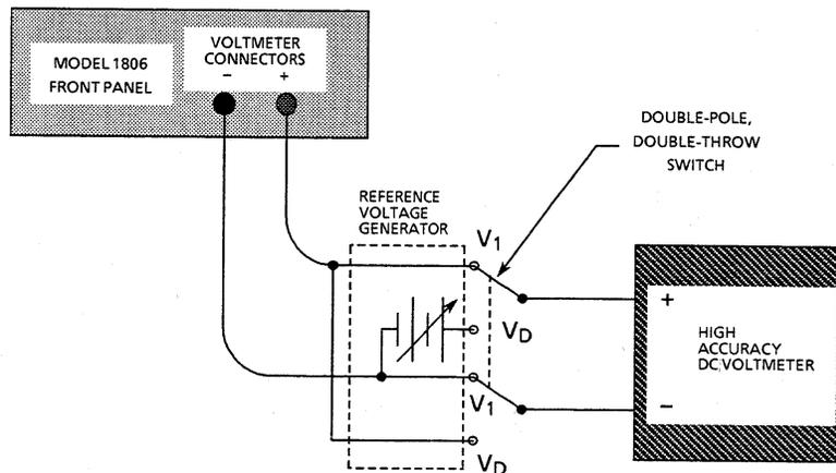
**Figure 3-3 Location of Reference Voltage Generator in Typical Test Configuration**
