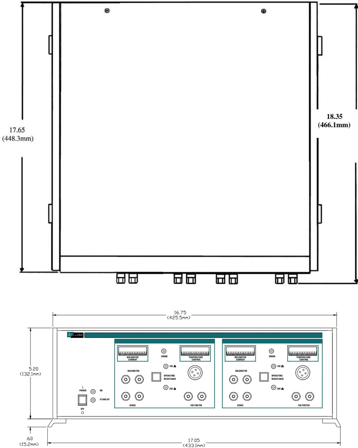
Figure 1-2 Model 1806 Dimensions (Top/Front)
