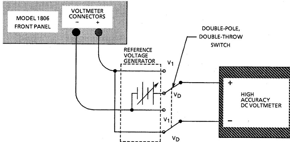
**Figure 4-4 Use of Reference Voltage Generator in Typical Test Configuration**
