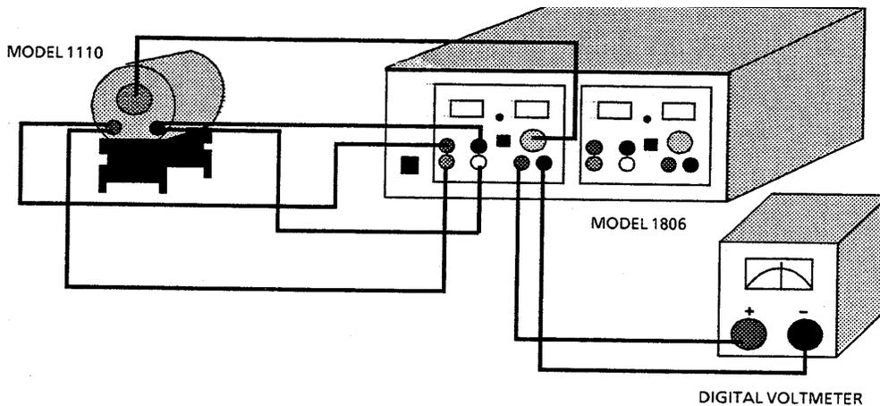
**Figure 5-4 Bridge Balance Test Configuration**
