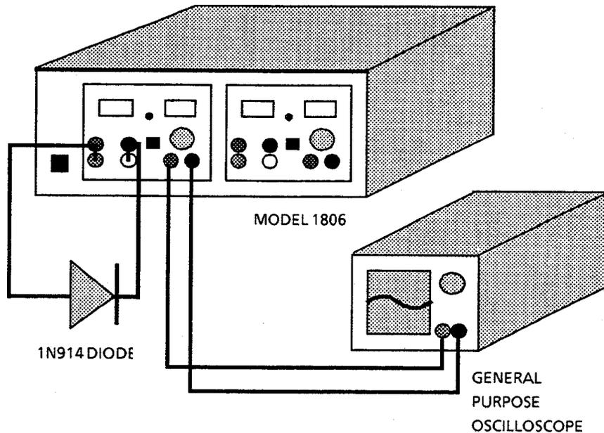
**Figure 5-3 Bridge Noise Test Configuration**
