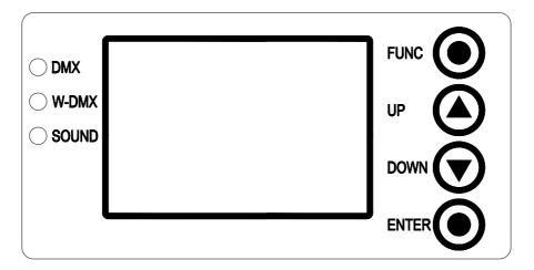
Fixture's address and function code configuration can be set conveniently via Touch Key and LCD display. Press button ENTER more than 3 seconds to unlock panel. LED display shows the fixture's function menu. Each Option of the main menu has its own sub-menu. Each menu stands for specified function of the fixture, please see the details in the following:
