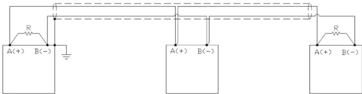
On the RS485 network normally one connects 2 termination resistors of 120 Ohm (shown with "R" in figure). Only on the 2 devices which are at the end of the network.
