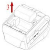
4. Detach the battery connector as shown in the figure on the right. Reverse Steps 1-4 to install the new battery pack.
