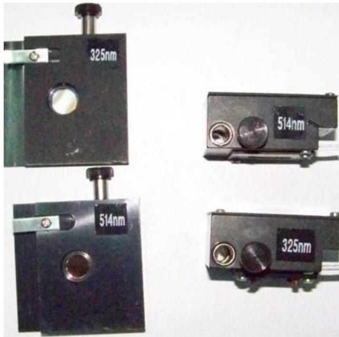
Fig.14 Lenses for Different LASER source
