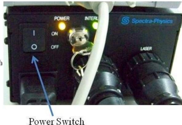
Fig.5 Power Unit for 514nm LASER
