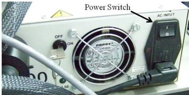
Fig.6 Power Unit for 325nm LASER
