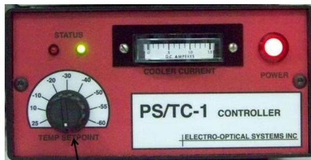
Fig.8 Temperature Controller for InGaAs Detector
