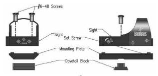
Kimber 1911s, Ruger Mark I, II, III, and compatible pistols Drive the rear sight out of its Dovetail Slot with a suitable drift pin (brass) or a fixture. Place the Sight on the Mounting Plate so that the screw holes in the Sight and Plate align. Press the four pins on the top of the Plate into the corresponding holes in the Sight. They do not need to be tightly together yet.
