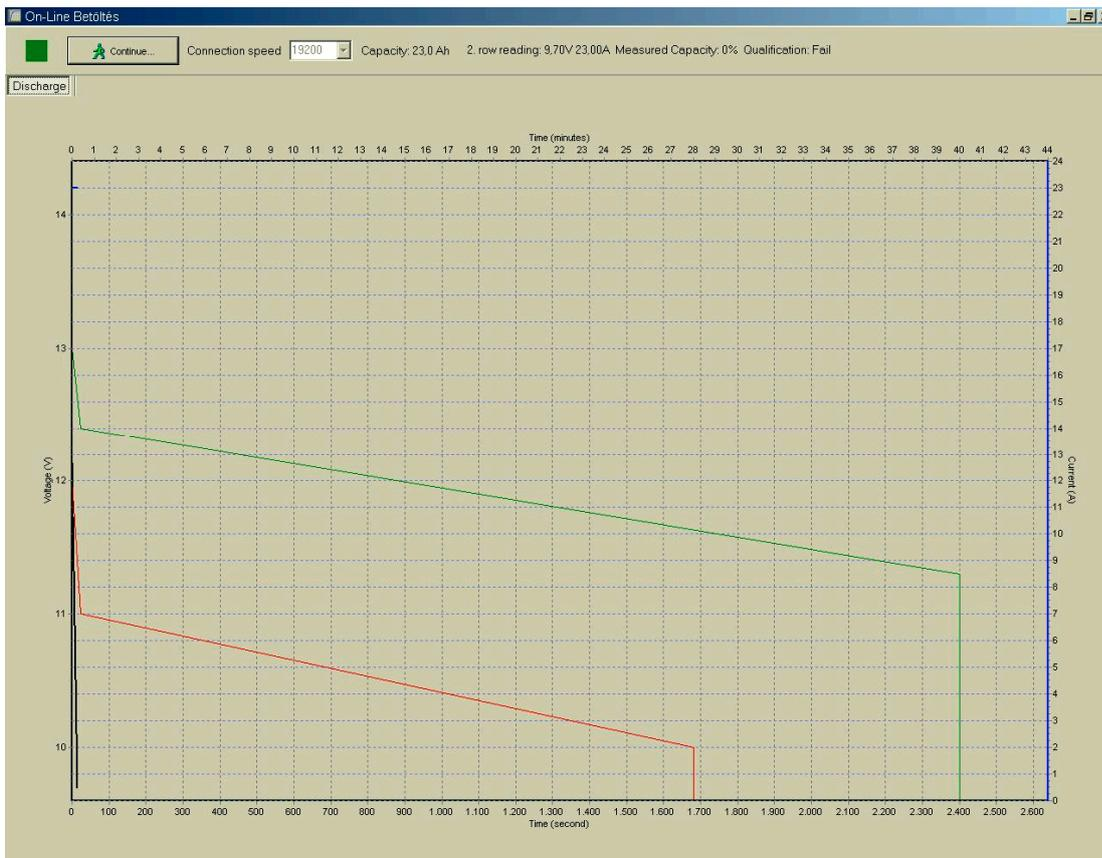
You see a green and a red line that shows the area between 60% and 100% capacity. The battery should be in between these two lines or above.
