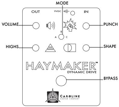
PUNCH controls the amount of drive. SHAPE is based on a mod Philip Ruetz shared with us; it sets the frequency response and overall grit or "hair" in the signal. HIGHS is a low-pass filter that manages the treble content. VOLUME adjusts the overall output.
