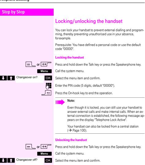
Enter the PIN code (5 digits, default "00000"). Press the On-hook key to end the operation.
