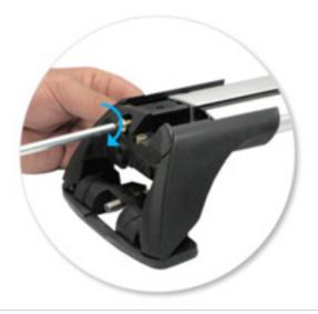
• Tighten adjusting screw to 5 Nm.
