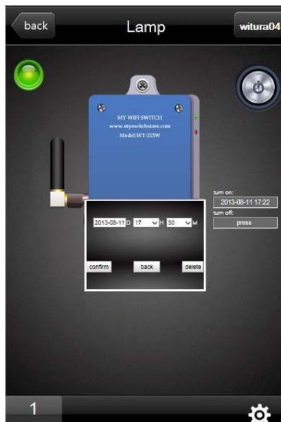
Fill up the **date, hours, minutes** column that you need to let the WT-215W to **Turn On**. Click the **confirm** button to confirm the Turn On time.
