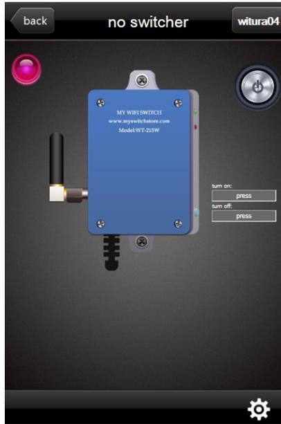
Go to the setting page to make the setting to connect the WT-215W, simply click the **setting** button at the right bottom button as shown on below;
