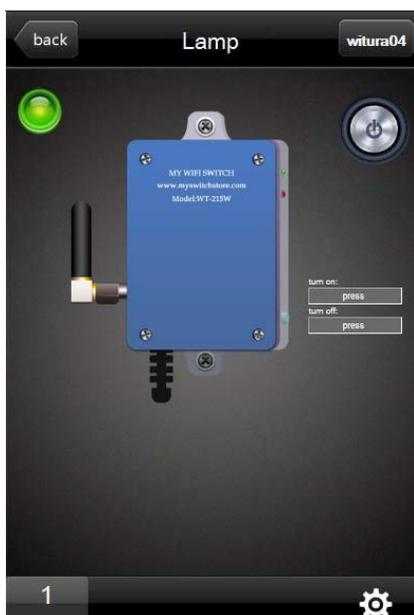
If the Light showing GREY colour as show below which means that the WIFI module is not online or not connected and you are not able to control the WIFI switch at this moment.
