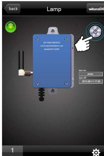
When reach the Turn Off time, the unit will Turn Off and you will see the light for the **power button** will switch off. As shown below;
