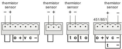
Note: The ±qdenotes the ground connection. This should be connected to the cable screen, if any.
