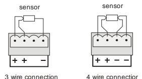
N.B. It is essential for 3 wire sensors that the resistances of all the connections are equal, i.e. the wires used for these connections should be of the same material, gauge and length. This allows the circuit to cancel the effects of lead resistance on the sensor measurement.
