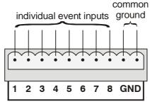
In both cases, if the maximum voltage could exceed 5V, then the addition of a 1K resistor in series with the input will allow voltages up to 6V to be used.
