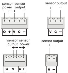
Note: if the cable used has an independent screen, this may be connected to the ground terminal, which is marked  $\mathfrak{D}q$
