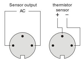
Note: the ±qconnection is ground and should be connected to the cable screen, if any.
