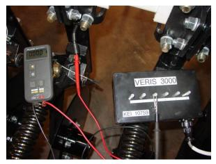
Figure 3.3 Testing cable at end of signal cable wiring harness
