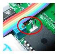
Figures 9.5 a, b, c 9a: Resistor installed for 2000XA and 3100 models; 9b and c: position for 3150 models: resistor in storage position—not being used; 9c resistor removed
