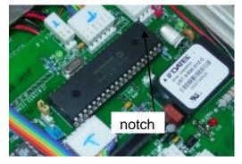
Figure 9.5 a and b. Notch on chip must be to the right, matching notch on chip socket
