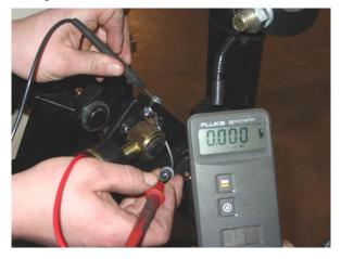
Figures 3.4 ab. a. Separating sure-seal connector b. Testing terminal connector wire
