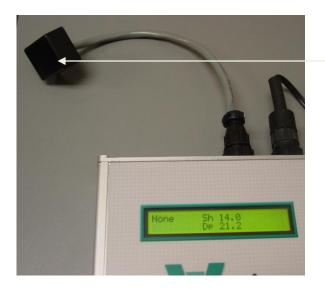
Signal Test Load
