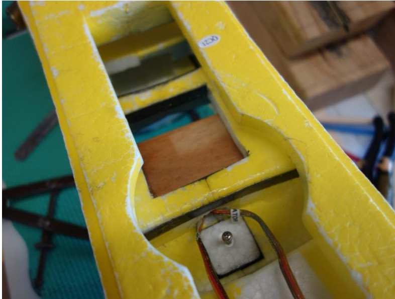
Opening in fuselage to allow easier access of cabling and better ventilation / air flow
