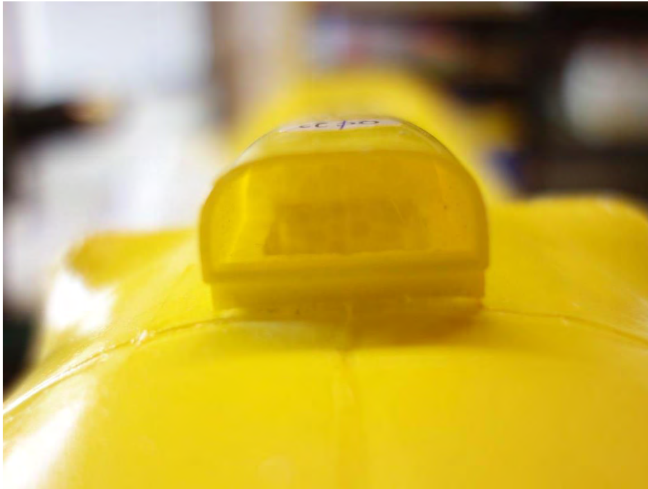
Lower inlet scoop opened up
