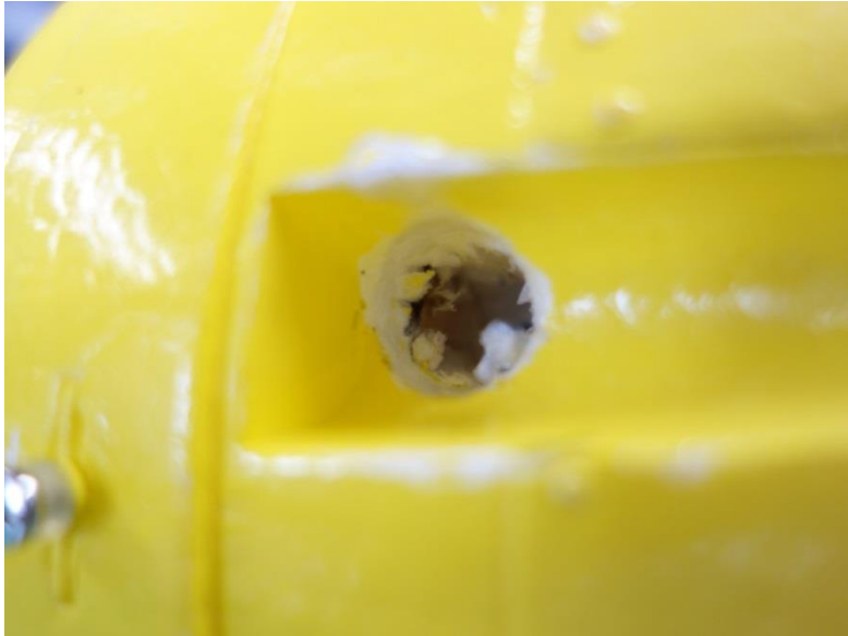
Opening in fuselage continued internally as to allow air flow from internal annular space immediately behind propeller
