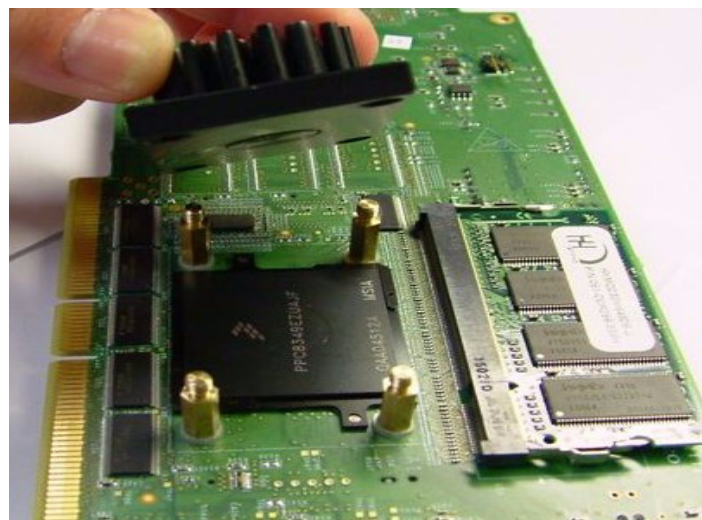
Figure 7-13. Remove heat sink
