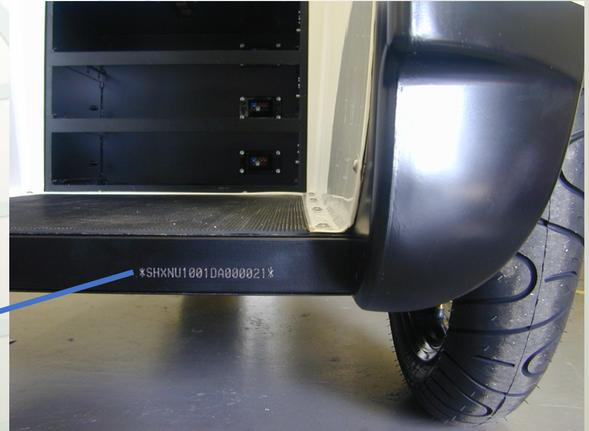
Location of VIN Number Stamped on Chassis
