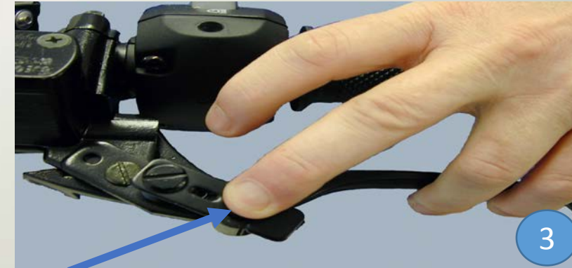
Whilst still applying brake and holding retainer back Push Pin Down The release retainer and brake
