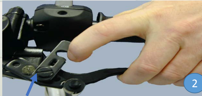
Slide Retainer back whilst still applying brake
